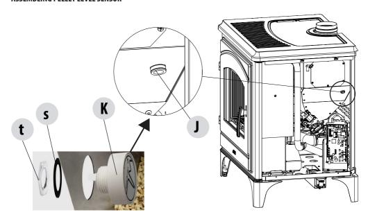
The pellet sensor is a low fuel indicator that warns the user that the pellets are finishing.
