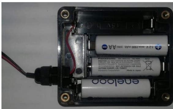
Fig. 18 – Replacing battery in battery box
