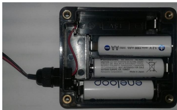
Fig. 21 – Replacing battery in battery box
