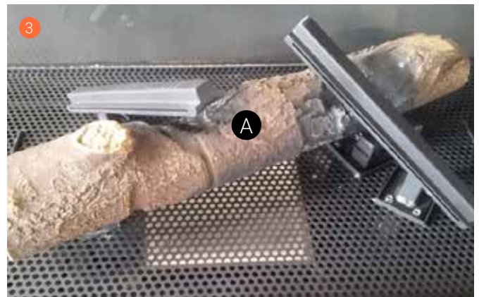
Push block A against the stop towards the pilot flame.
