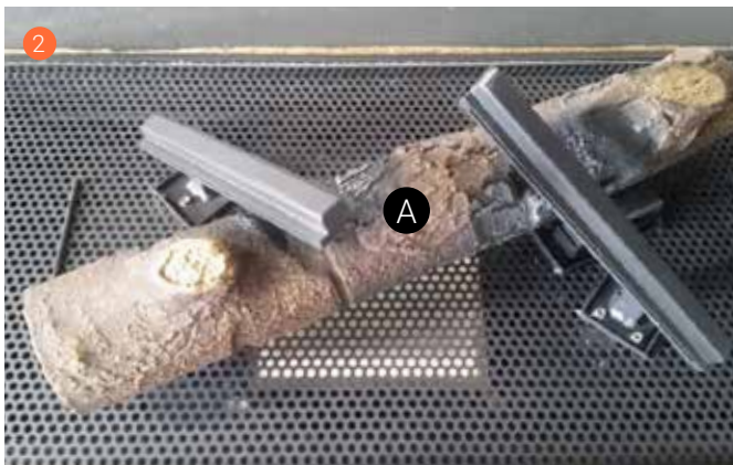
Disassemble one of the standing burners to install block A.
