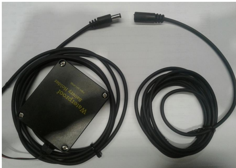
Photo 14 – Battery box connection
