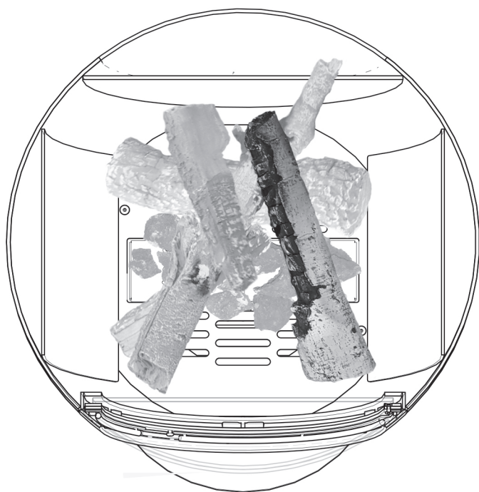
Position Log G6 as shown in the diagram. Scatter the Glow Strands among the Logs and Embers. Finally Check the appliance for Pilot ignition and cross lighting ensuring that no material is impinging the operation of the Pilot.
