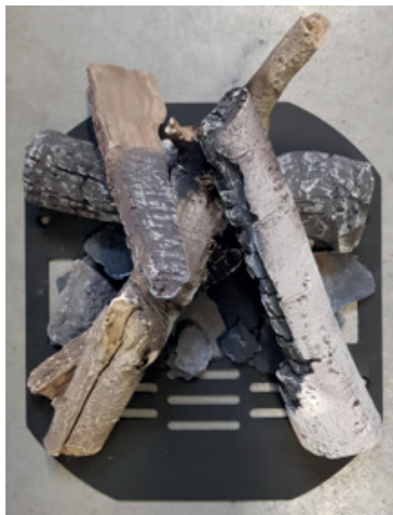
Position Log G6 as shown in the diagram. Scatter the Glow Strands among the Logs and Embers. Finally Check the appliance for Pilot ignition and cross lighting ensuring that no material is impinging the operation of the Pilot.
