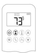
To change between °C and °F, press <sup>(1)</sup> and <sup>(2)</sup> buttons simultaneously.
