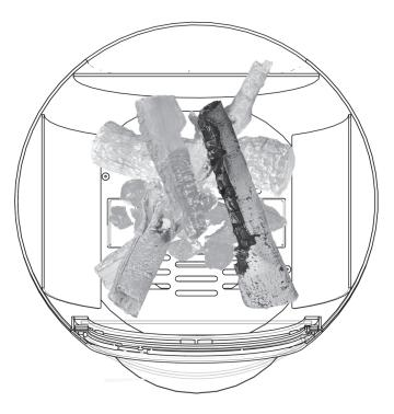
Position Log G6 as shown in the diagram. Scatter the Glow Strands among the Logs and Embers. Finaly Check the appliance for Pilot ignition and cross lighting ensuring that no material is impinginging the operation of the Pilot.
