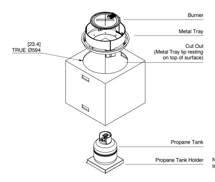
NOTE: Retention means must be provided to limit the movement of the LP gas cylinder.
