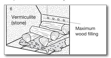
The fuel load, must be maintained below the top series of air holes and within the outer vent in each side. Fig. 6.
