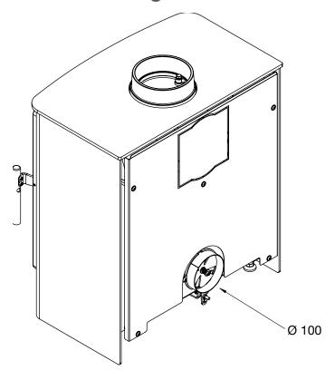
When installing external air supply, connect the air intake to the direct air pipe using flexi-pipe,
